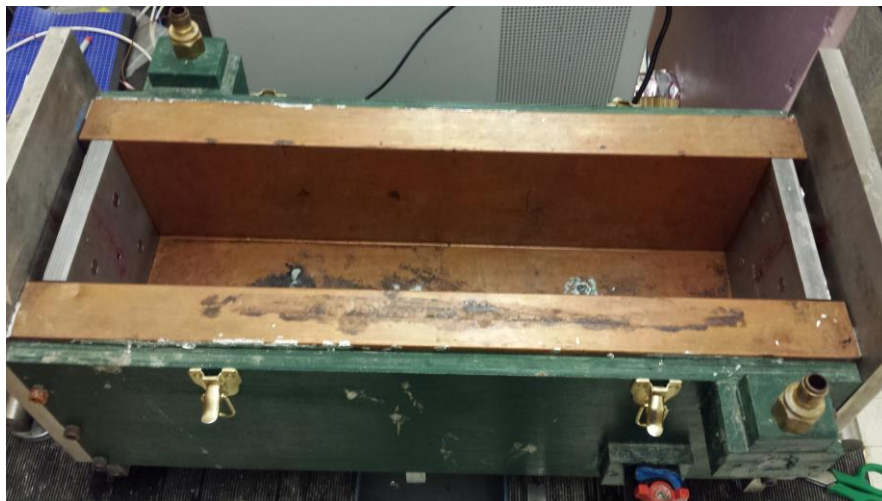
Figure 3 Free shrinkage frame empty
