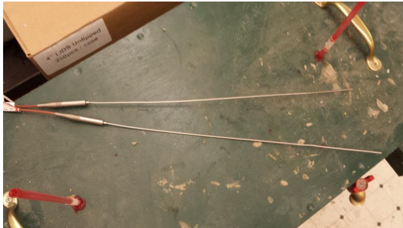
Figure 6 Type T stainless steel thermocouples used to determine the temperature of the concrete in the free shrinkage frame
