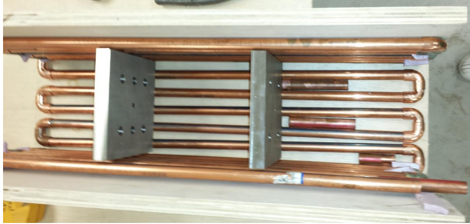
Figure A.1 The copper piping that circulates the coolant fluid. The pipes are numerous and as tight as can be to maximize surface area
