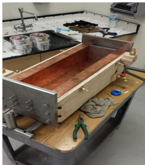
Figure A.9 Finishing touches of the construction of the free shrinkage frame. This includes a drain for easy emptying of the frame and latches for a good seal during operation
