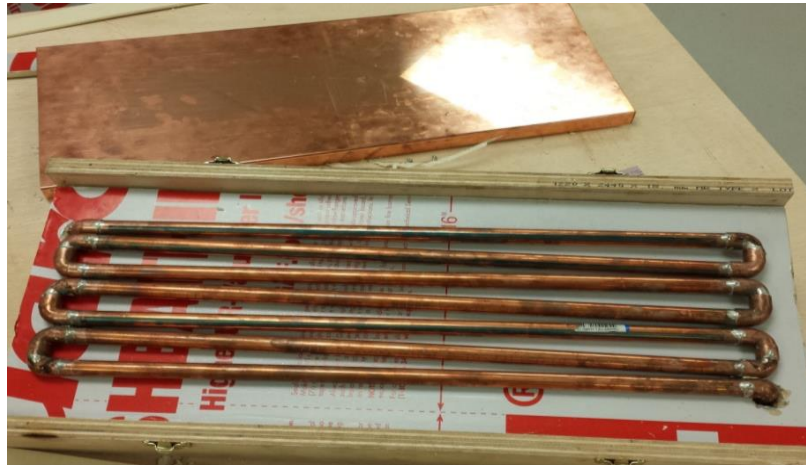
Figure A.8 Pipe layout and copper plate before finalizing the construction of the free shrinkage frame lid
